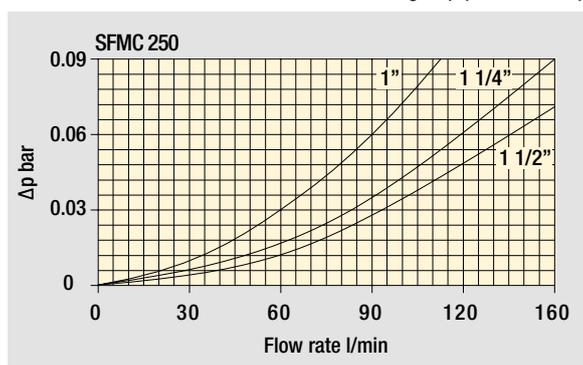
Bypass valve pressure drop
