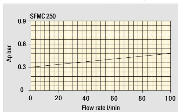
The curves are plotted using mineral oil with density of 0.86 kg/dm<sup>3</sup> in compliance with ISO 3968.  $\Delta p$  varies proportionally with density.
