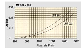
Bypass valve pressure drop
