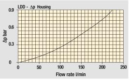
Bypass valve pressure drop
